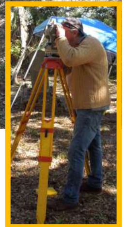
Above and right: Caitlyn Johnson holds a prism pole steady while Ken Sassaman aims the laser total station. Both marked and unmarked graves were mapped and coded accordingly.
