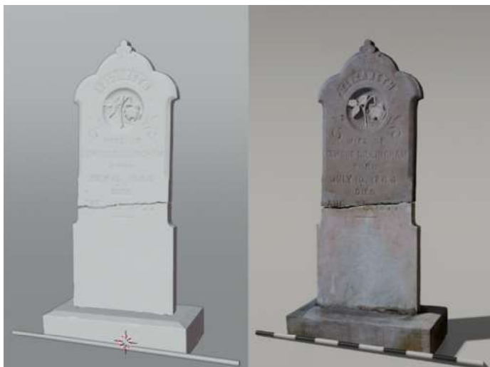
Above: The headstone of Elizabeth Dillingham as reconstructed using 3D photogrammetry.
