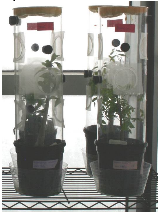
Figure B. Plexiglas cylinders (45 cm x 15 cm diameter) used to conduct no-choice tests for the thrips Pseudophilothrips ichini .
